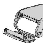
3. Holding the free end of the paper and the terminal, close the printer cover and push firmly until it locks.
